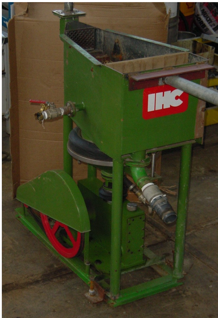
Figure 3: A through-screen discharge jig as used for valuable minerals concentration
